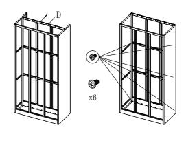
4: Installing the G to the cabinet, pay attention to the screws installed
