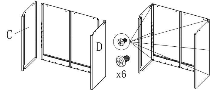
3. Shown mounted with screws E, F to C, D on
