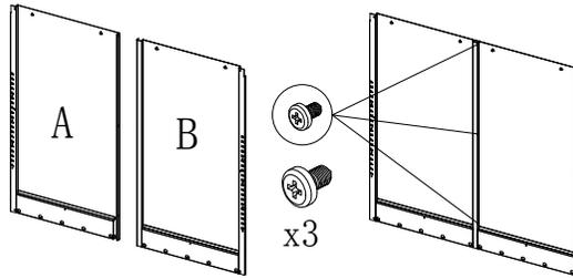
2. Mounted with screws C, D to A, B on
