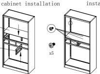
5. Figure installing J, then install the I to the cabinet
