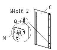
2: The B, C mounting onto A, with P fixed
