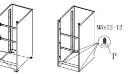
6: As shown installed rails L, G locks (When installing G, there is a note that locks the arrow side up, the rotational direction of the latch is shown below)
