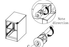
c:As the L mounted to the drawer, and with T connection U, H, J
