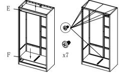
4: Mounting direction shown in FIG. G, and screw Fixed
