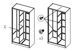
5: Respectively mounted L, H, I to the cabinet with screws Fixed, as shown below
