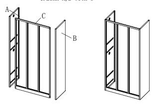
2. Connect D and A, B, and fixed with screws
