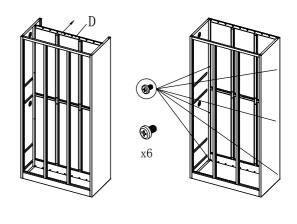
5. Installing the  $\ensuremath{\mathsf{G}}$  to the cabinet, and secure with screws
