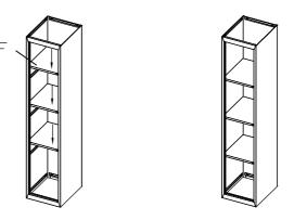
5. Attached to the H on G, then G were installed from the bottom up
