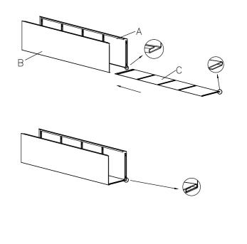
2. Installing the D to the cabinet
