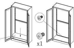
5. Figure installing G, pay attention to adjust spacing
