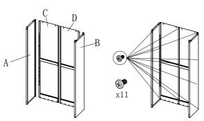
2.Link E with A,B fix by screws
