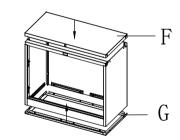
8. Install the assembled drawer cabinet and fitted with M and N
