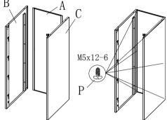
2: The B, C mounting onto A, with P fixed
