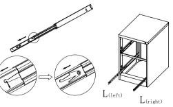
7: Packed onto the drawer on the cabinet (installed)
